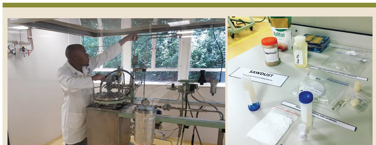
**ABOVE:** Pule Seemela, a technician in the BDF, operating a flow-through digester.
