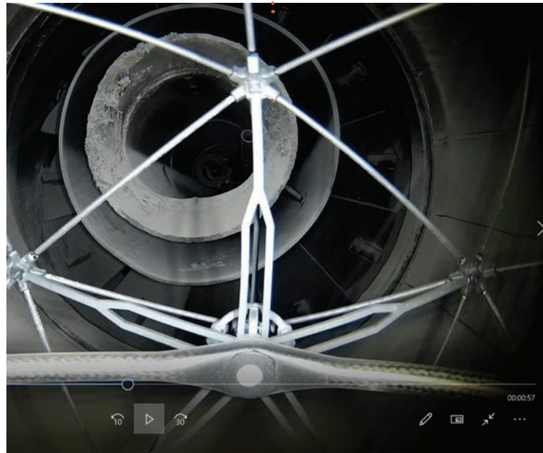
TOP: The Elios collision-tolerant drone is the latest hi-tech inspection technology from Skyriders. BELOW: Flying from chamber to chamber, the drone picks up any irregularities on the screen.
