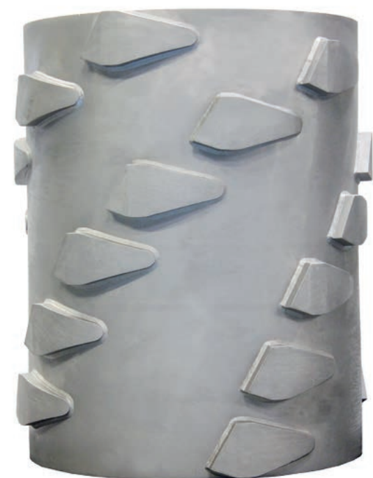
FIGURE 4. DRUM 450 Dolphin rotor for coarse screening. The rotor creates optimal pressure pulses (positive pulse for debris removal efficiency and negative pulse for cleaning to minimise plugging).
