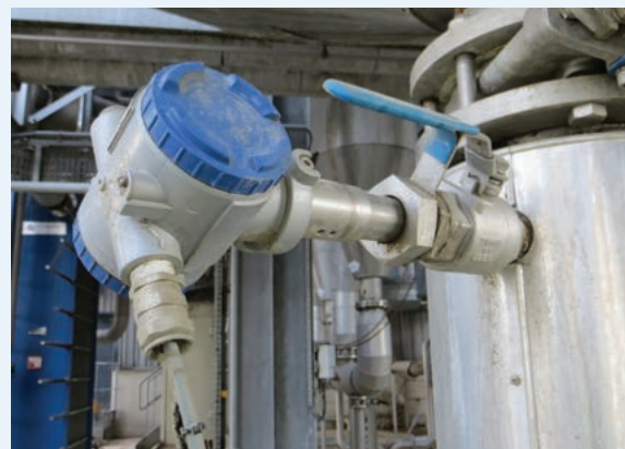
Fuji level and pressure transmitters with ball valve design at Cristal Union's manufacturing plant in Aulnat, central France. Maintenance teams don't have to take the tank out of service to remove the transmitter for maintenance.
