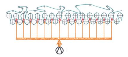
(TOP) **FIGURE 1**: Unfavourable – "undercurrent". (BOTTOM) **FIGURE 2**: Very good – blow pipes distribute air in a sensible and directed way
