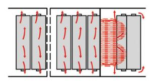
(LEFT) **FIGURE 3.** Optimally placed blow pipe. (ABOVE) **FIGURE 4.** Recommended air flow from the pockets. (BELOW) **FIGURE 5.** Uneven pocket ventilation = uneven moisture removal.
