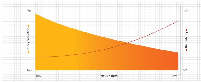
(ABOVE) FIGURE 1: Effect of the profile height on sticky reduction and on runnability. (RIGHT) FIGURE 2: Pilot Plant Results
