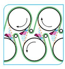
(LEFT) **FIGURE 6.** Even pocket ventilation – regularity across the board. (RIGHT) **FIGURE 7.** Air doctors in cross section
