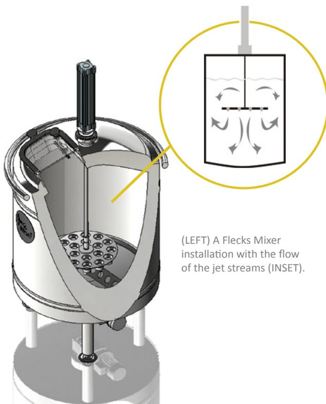
(LEFT) A Flecks Mixer installation with the flow of the jet streams (INSET).
