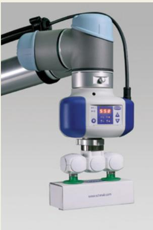
The electrical vacuum generator ECBP from Schmalz with intelligent interface for connection with grippers and robots.
