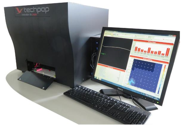
The chemical nature of stickies makes them suitable for analysis by near-infrared spectroscopy (NIRS). The technique is rapidly gaining acceptance in the industry, with applications in paper recycling such as paper waste stream sorting<sup>[2,3,4]</sup>, raw material quality assessment<sup>[5,6,7]</sup> or quantification of stickies embedded in handsheets<sup>[8,9]</sup>.
